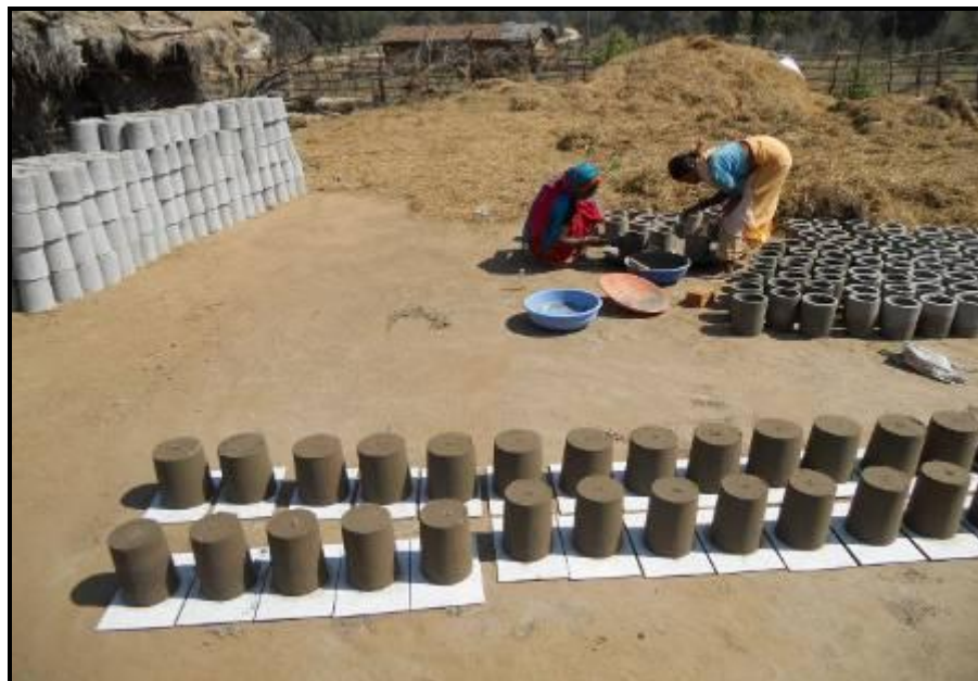
SHG Members are preparing in cement layering of Pitcher.
